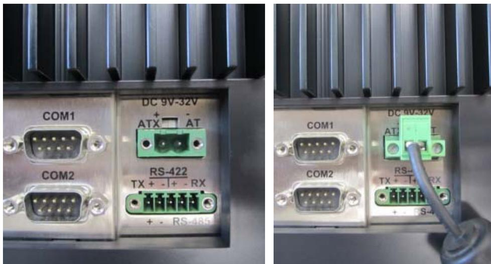
Figure 2.4 Connect Power Cable
